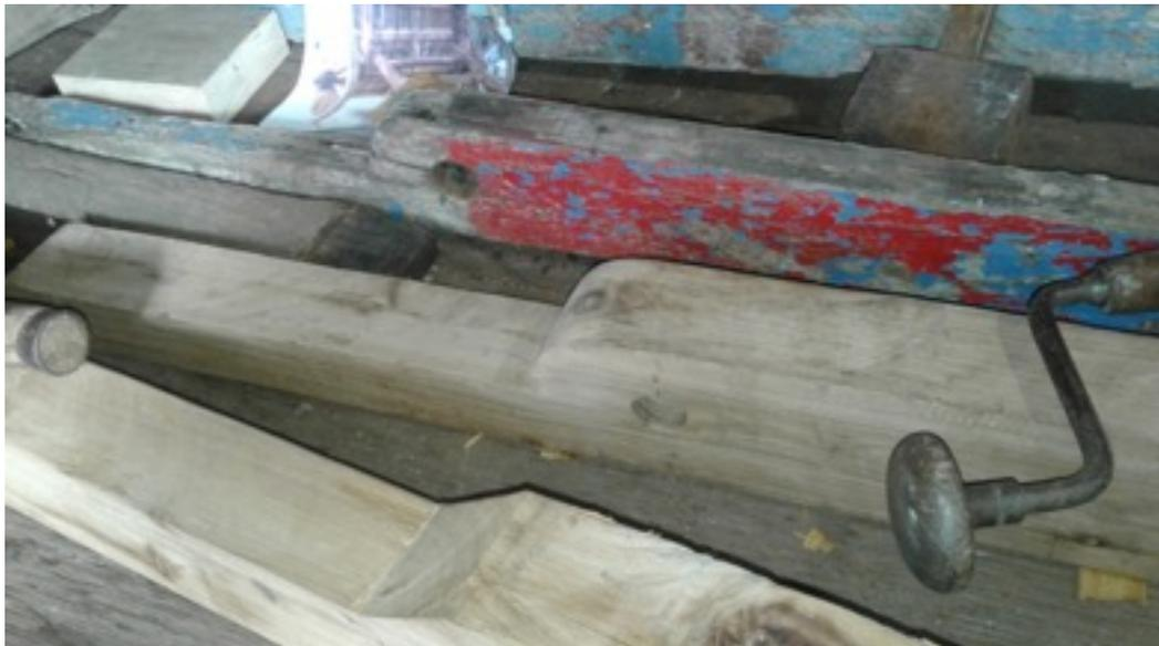
In the centre you can see the old part with the paint, and the new wider one just about completed. Of Course the old dray was built to Imperial measure (feet and inches) and the metric timber had to be cut down to original dimensions to fit the old metal parts, and be faithful to the original.
