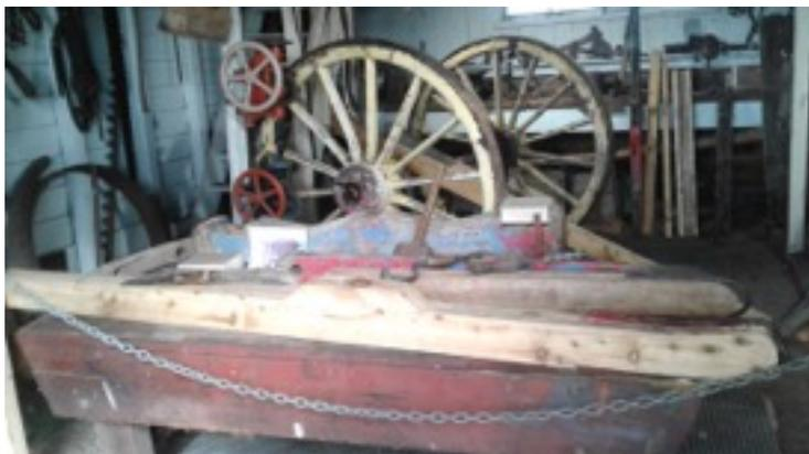
Roughed out parts of the tipping section are already in the Amess Barn, our working space, awaiting adaption to existing metal fittings and recreation of others by the Island's Blacksmith. The wheels were in a sad state and only suitable for static display under cover but FOCIS has sourced similar aged wheels in excellent condition and is awaiting some work by an outside firm to detach them from another construction.
